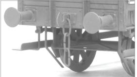
hole in the coupling hook. I reinforce the joint of each link with a spot of 60/40 solder.
