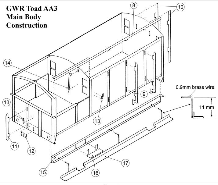
3. Emboss rivet heads into top strips (parts 8) and then fold the end section to form a 90 degree angle. Then locate the strips into the etched rebates along the top of the sides with the end of the angle section fitting behind the corner plate of the veranda end. It may be necessary to file the end of the strip slightly to achieve a snug fit as you don't want the strip to push the top of the veranda end outwards.
