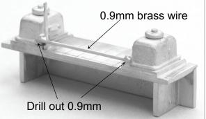
Fit the etched operating handle (part 24) hard up against the brass wire and right hand sandbox. Then fit the sandbox/locker casting into the veranda hard against the veranda end (you should be able to trim the tags of the end stanchions flush with side cutters) You may have to file the ends of the locker casting to achieve a snug fit.
